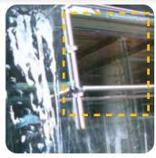
**After:** A section at the top right of the panel was easily cleaned after 4 months, showing no signs of etching.
